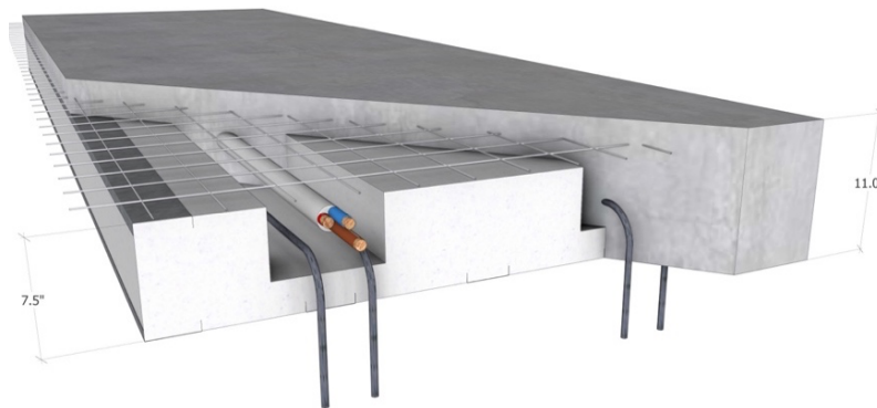
Fig 1: fpanel general view geometry and stud's locations
