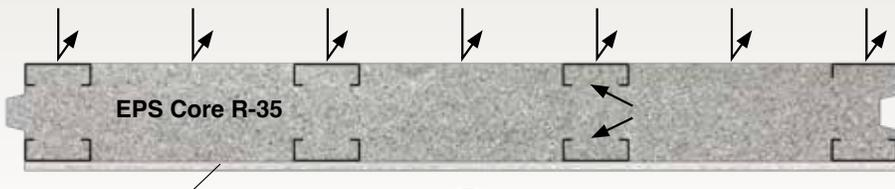
Tabbed connection to next panel with self-drilling screws.
