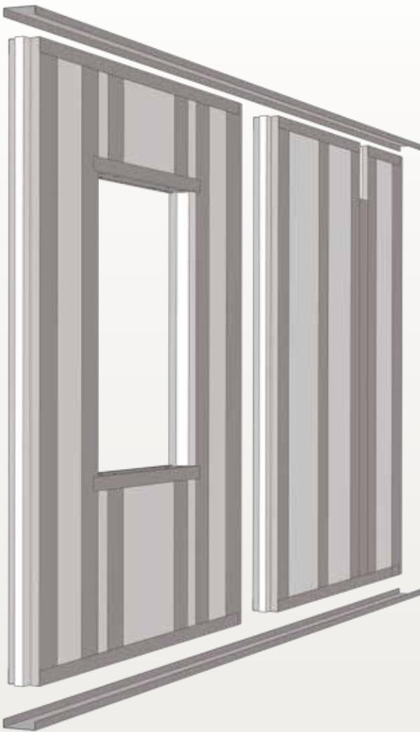
Example shows typical window rough opening, beam pocket, and top and bottom track.
