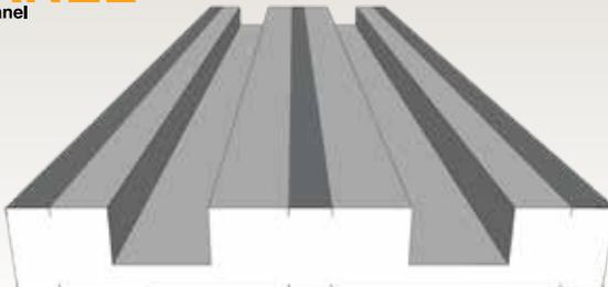
**fPanel** - 48" Max width, 144" max length. Panels connect end-to-end and side-to-side for coverage. Rebar troughs to form grade beams, top with rebar mesh and 3-4" concrete. Panels connect end to end and side to side for coverage.
