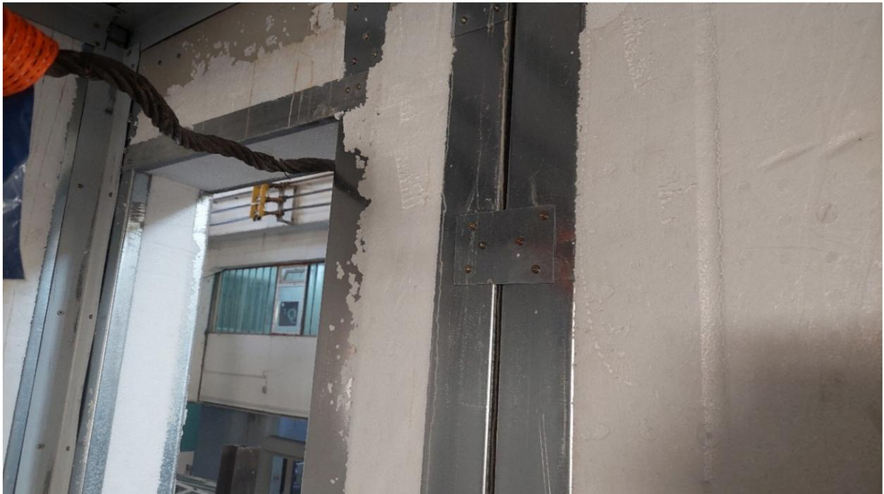
*Fig. 33 Interior connector and window opening detail on wall B – structural model THS 24-388 after completion of the tests.*
