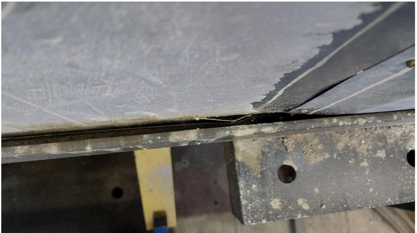
Fig. 45 Detail of the base area of wall A – structural model THS 24-389 after completion of the tests.
