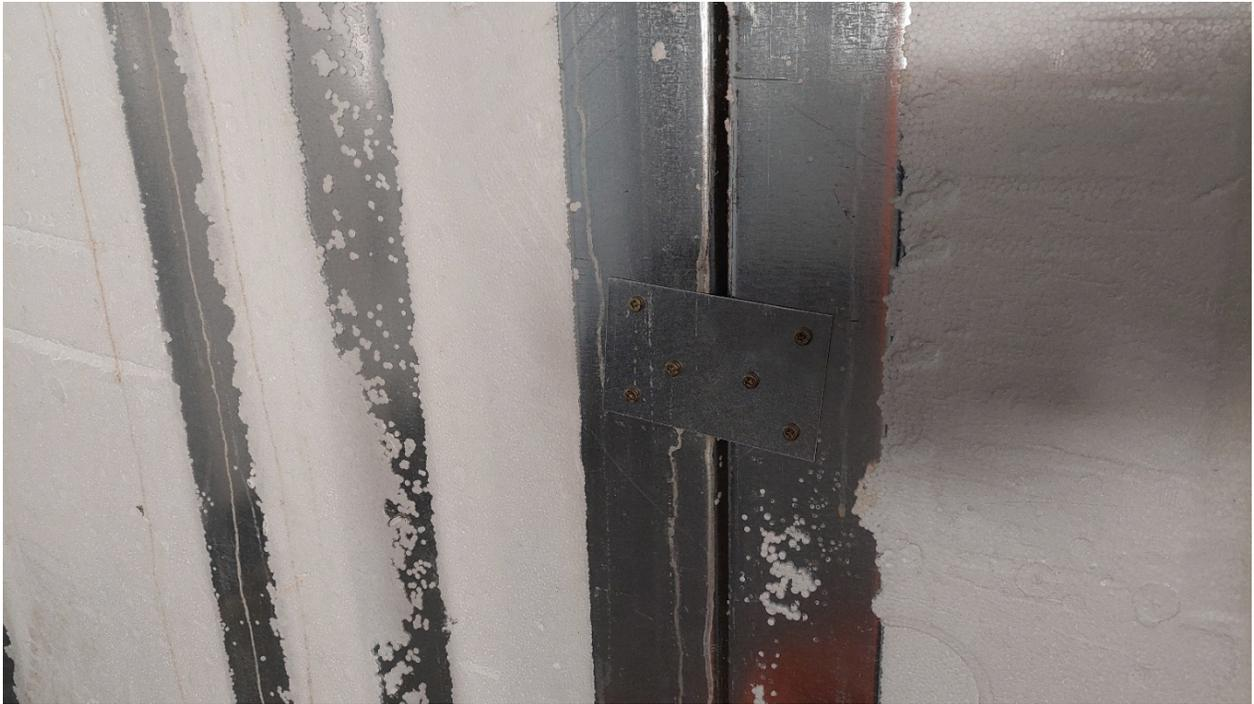
*Fig. 32 Interior connector detail on wall B – structural model THS 24-388 after completion of the tests.*
