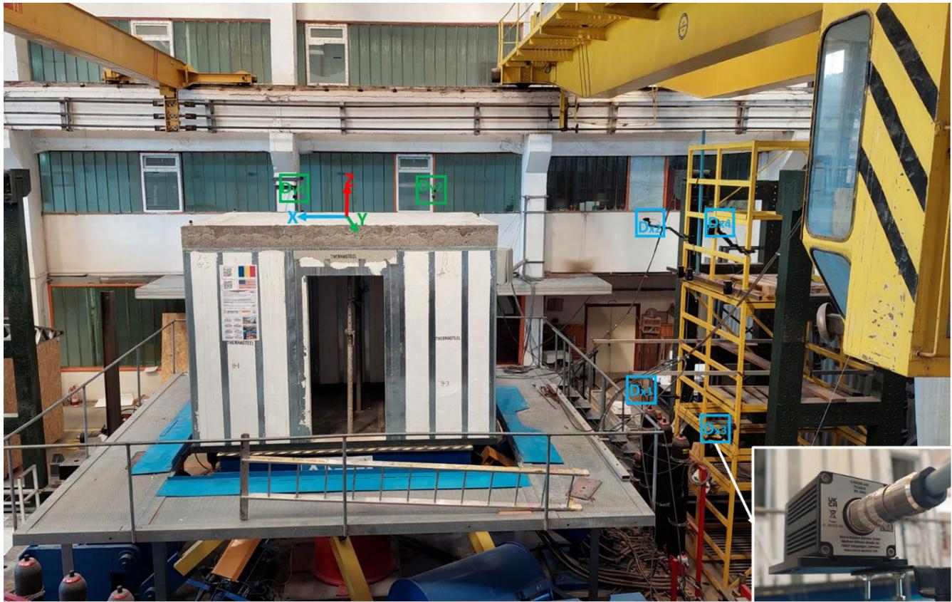
Fig. 17 – Position of LASER displacement transducers on the structure
