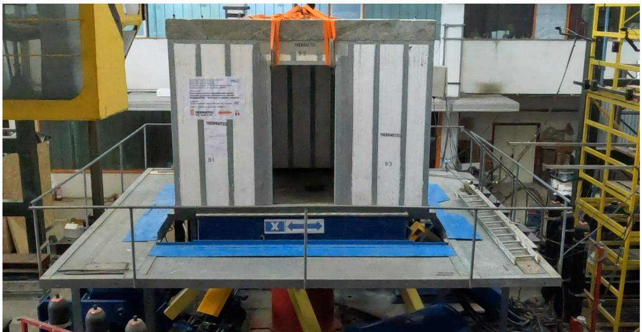
Fig. 2 – Structural model with *THERMASTEEL* panels – THS 24-389 (steel 1.09 mm, EPS 16.9 kg/m<sup>3</sup>)
