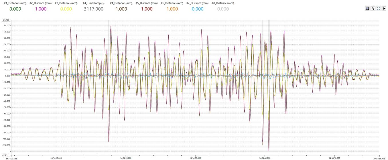
Fig. 23 Absolute displacement–time plots in the X and Y directions for action - Artificial 5 scaled 100%.
