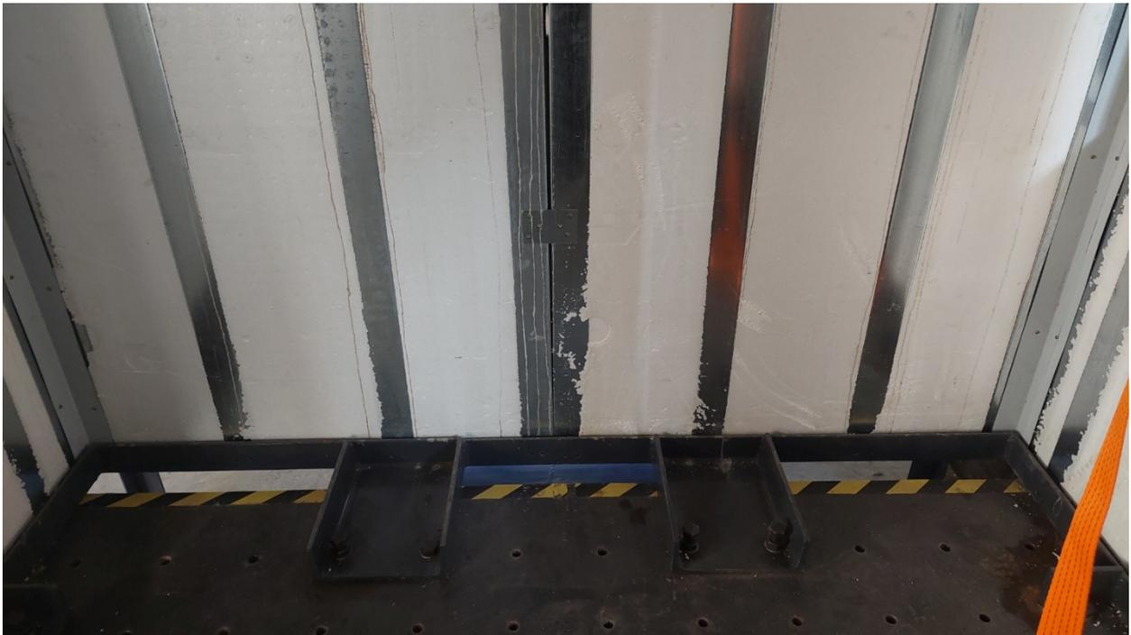
Fig. 31 Interior detail, base of walls B and 1 – structural model THS 24-388 after completion of the tests.
