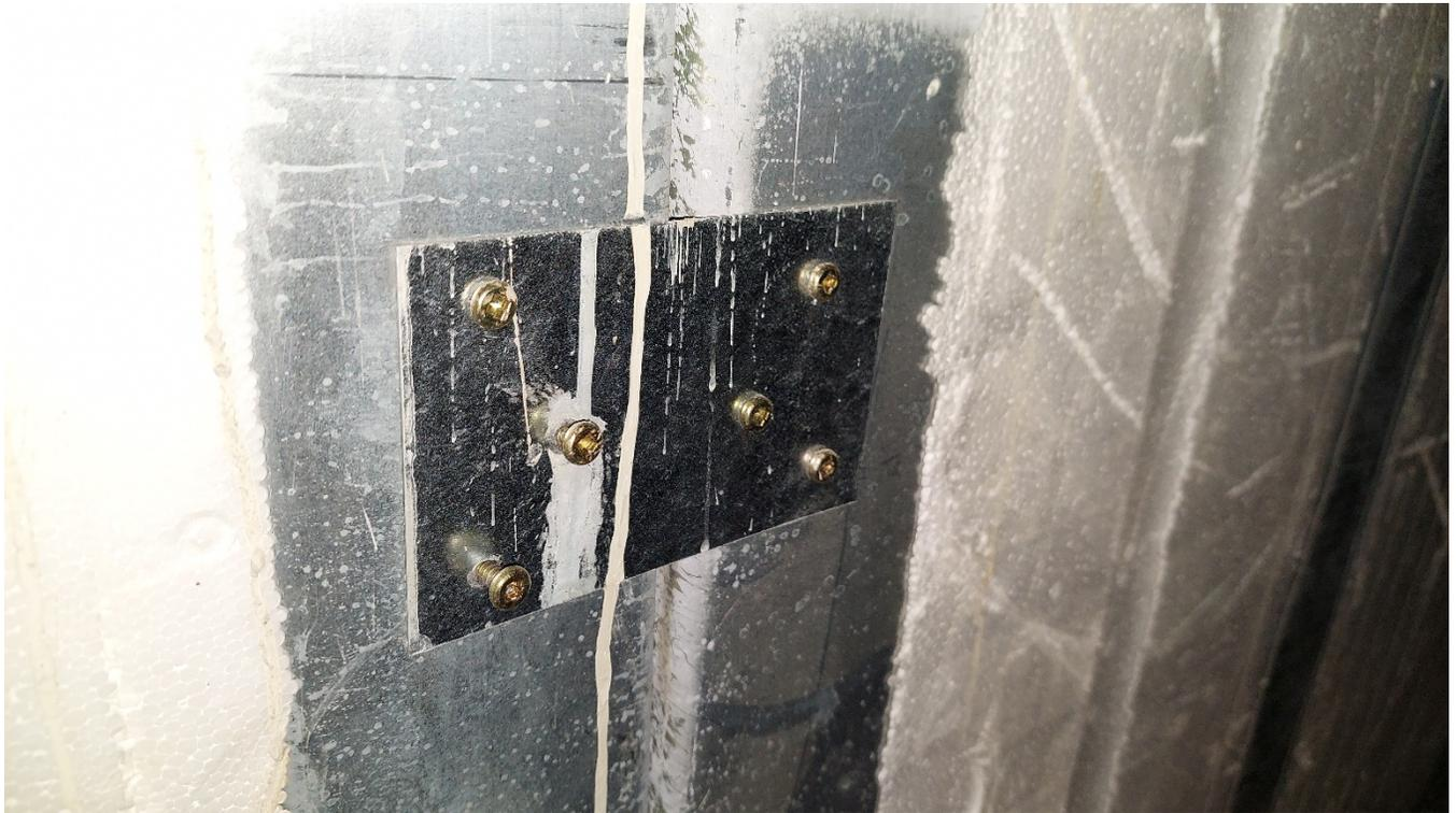
*Fig. 36 Lower joint between panels on wall A (interior view) – structural model THS 24-389 after completion of the tests.*
