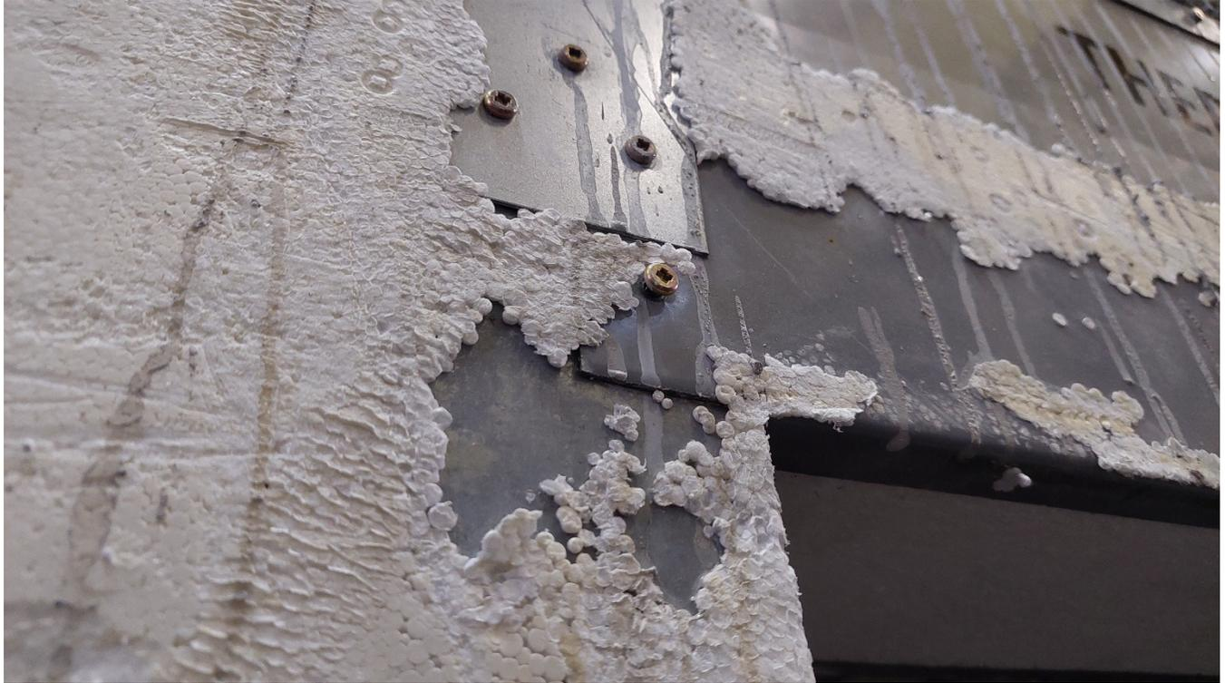
*Fig. 41 Door opening detail on wall B after action Artificial 1 scaled to 80% – structural model THS 24-389.*
