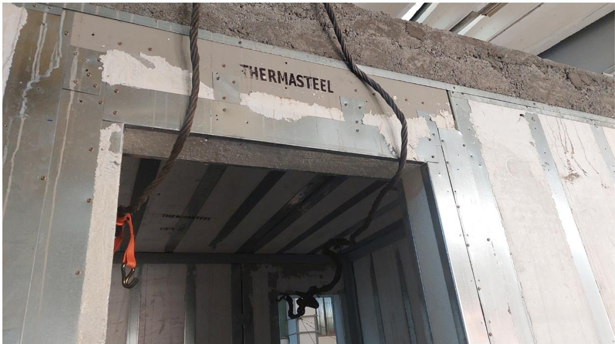
Fig. 27 Window opening detail on wall A – structural model THS 24-388 after completion of the tests.
