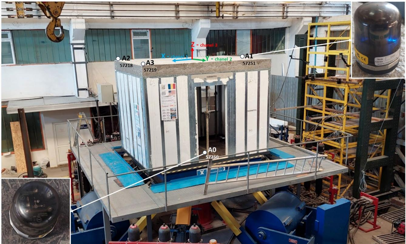
Fig. 16 – Position of accelerometers on the structure
