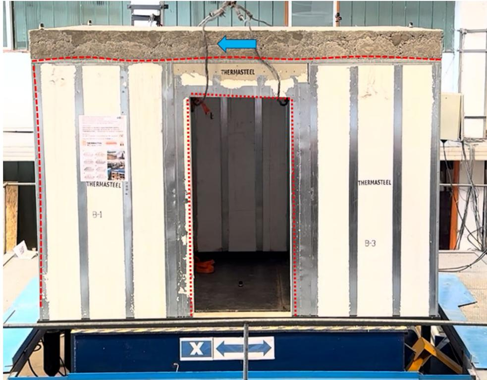
Fig. 34 Video frame detail of wall B, model THS 24-388, during the Turkey 2023 action – motion to the left.
