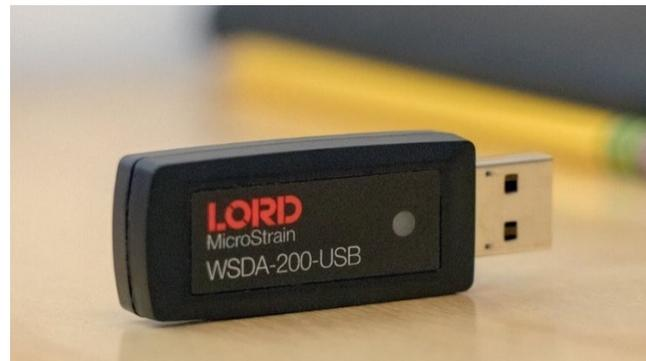
Fig. 9b- Data acquisition system WSDA-200-USB Wireless Gateway
