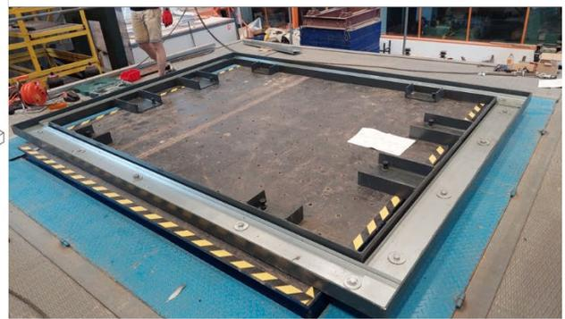
Fig. 3 – Adapter base frame made of UPN 300 channels and installation of the THERMASTEEL U-track (190 mm)
