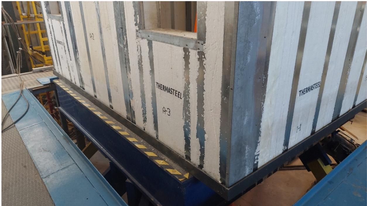
Fig. 26 Lower part of wall A – structural model THS 24-388 after completion of the tests.
