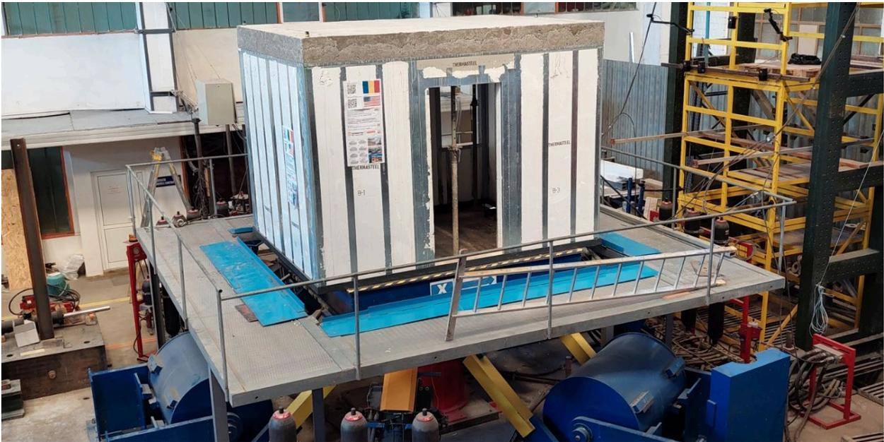
Fig. 1 – Structural model with *THERMASTEEL* panels – THS 24-388 (steel 0.84 mm, EPS 24 kg/m<sup>3</sup>), full-scale assembled
