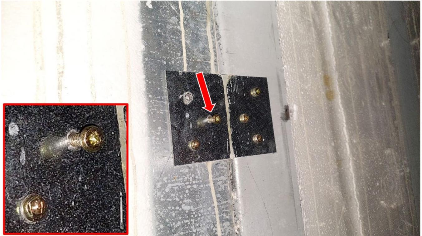
Fig. 37 Upper joint between panels on wall A (exterior view) – structural model THS 24-389 after completion of the tests.
