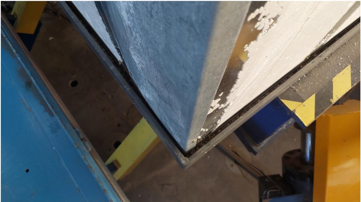
*Fig. 29 Exterior corner base detail between walls B and 1 – structural model THS 24-388 after completion of the tests.*
