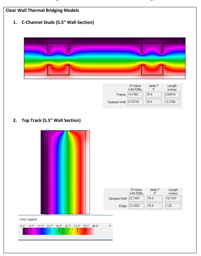
Table 1: U-factor Calculation for 5.5" ThermaSteel Panel Wall
