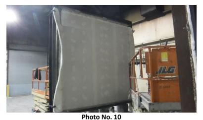
Third Layer Vertical Orientation Gypsum Installed and Ready to Test (Unexposed Face)
